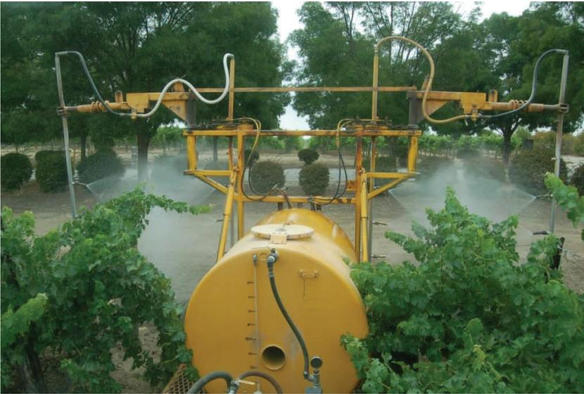
Figure 3. Commercial tractor sprayer used for large plot trial
