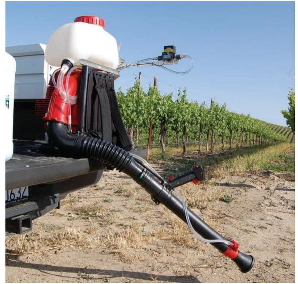
Figure 4. Backpack mist blower used for small plot trial
