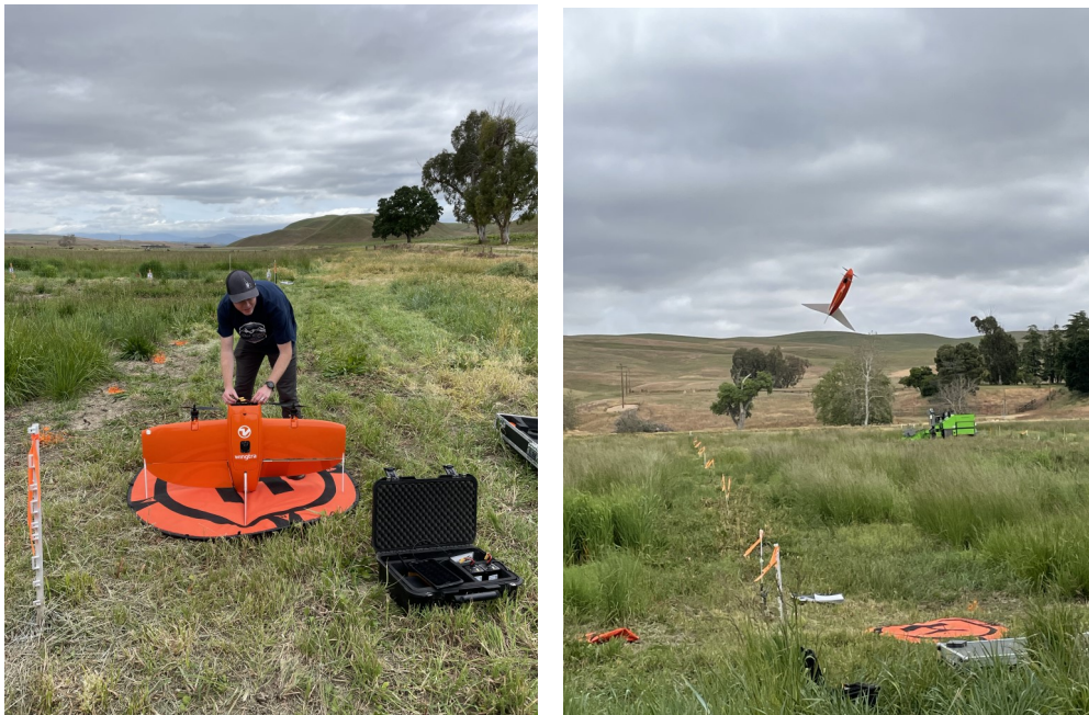
Setting up and launching a Wingtra II fixed-wing aircraft integrated with a Sony RX1 RGB camera.
