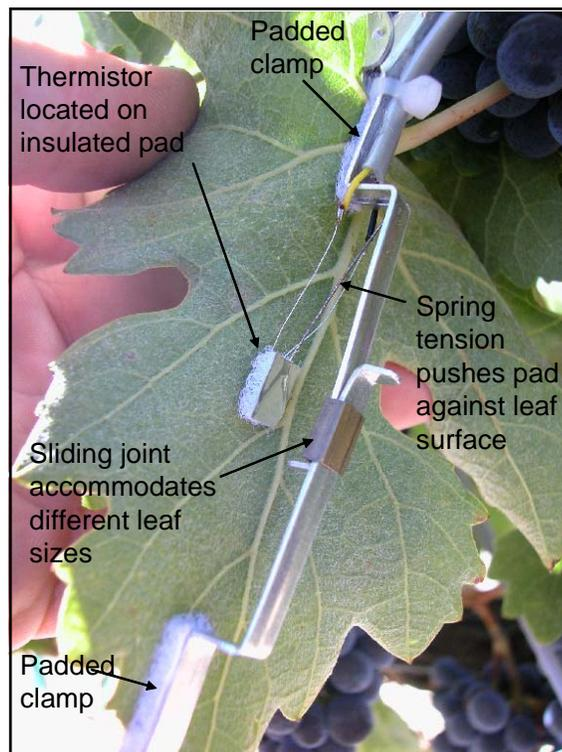
Figure 1. View of the leaf temperature sensor from the underside of the leaf. The thermistor is about the size of a pinhead, and is kept in constant contact with the underside of the leaf blade.
