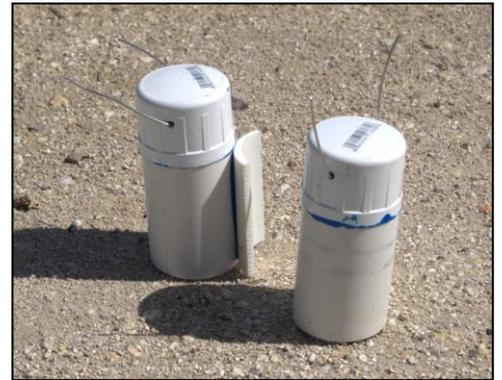
Program each "Hobo Pendant" datalogger to measure temperature at 5-minute intervals; use the "delayed start" option to synchronize their measurement times. Insert the dataloggers into the prepared radiation shields, and use the wire to secure them in place.
