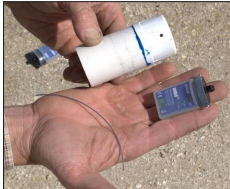
In this example, the shield for the lower datalogger has an additional "saddle" piece made from 1-1/2" PVC pipe glued to the side; this may help it attach more securely to the line post. This is optional.
