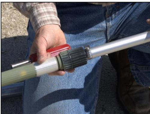
Fully extend the lower extendible aluminum pole section from the “Mr. Longarm.” Once fully extended, retract it one foot back inside the fiberglass section. This is important to do, as it provides additional support at this weak point. Tighten the black plastic lock by hand.
